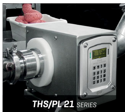
INTEGRATED SYSTEM WITH METAL DETECTOR FOR LIQUID AND VISCIOUS PRODUCTS
