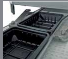
Fast, reliable denesting at 120+ trays per minute
