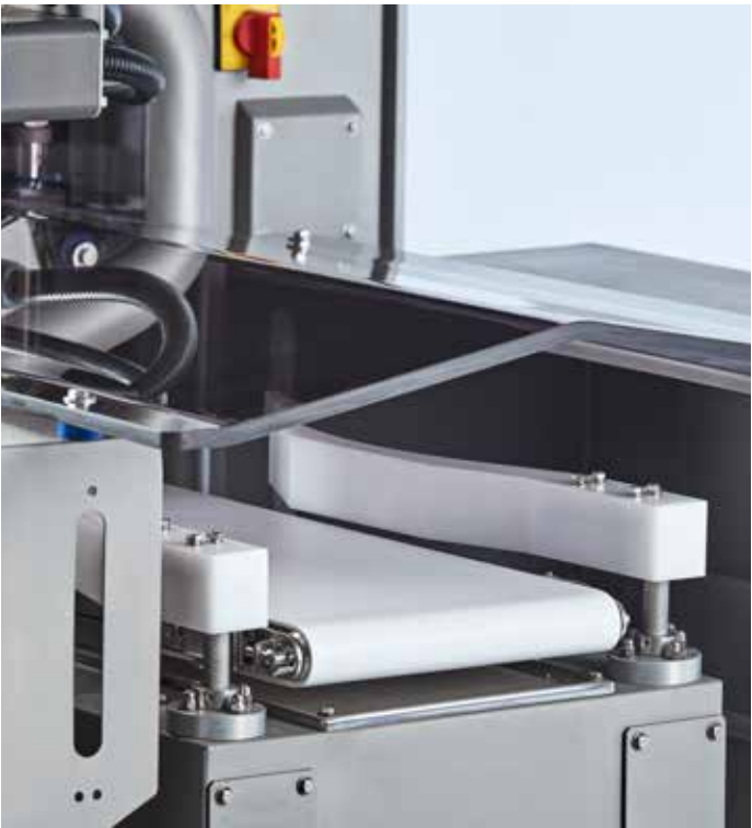
Catch arm rejects on seal tester
